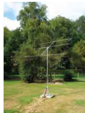
Top: Transmitter located in Dourbes (a crossed dipole with a 8m x 8m metallic grid acting as a reflecting plan). Left: Receiving antenna located in Uccle (3-elements Yagi antenna).
