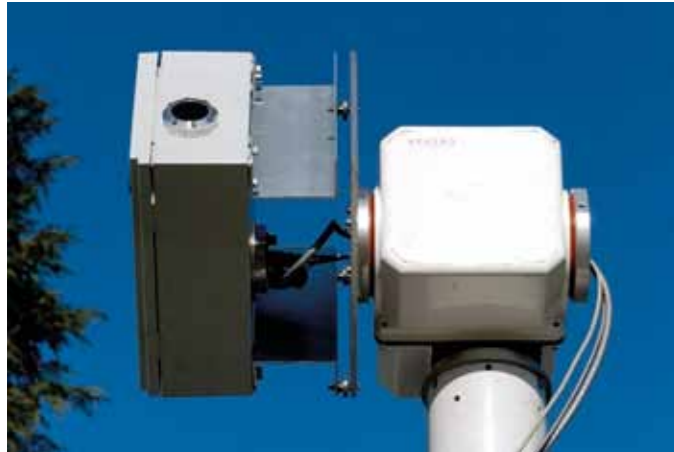
BIRA-IASB MAXDOAS instrument. The optical head is mounted on a sun tracking system allowing for alternate direct-sun and elevation scan measurement sequences.
