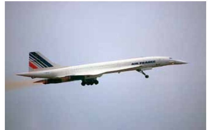
Take-off of a Concorde during a commercial flight, the exhaust clearly shows a red trail due to the instantaneous transformation of nitrogen monoxide to nitrogen dioxide on the surface. This high production of nitrogen oxides reflects the very high efficiency of the Concorde engines. (credit: Philippe Noret)
