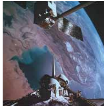
Deployment of the EURECA satellite with the help of the Remote Manipulator System arm. (credit: NASA)
