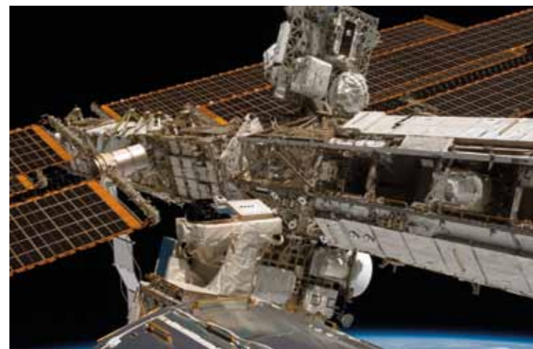
SOLSPEC (at the centre with the four holes) integrated in the SOLAR platform mounted on the exterior of the European Columbus module of the International Space Station (ISS). (credit: ESA/NASA)
