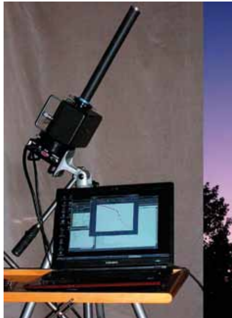
The Charge-Coupled Device (CCD) spectrometer used for measurements and the twilight sky above Tbilisi at the solar zenith angle about 93° colored after the Nabro eruption.
