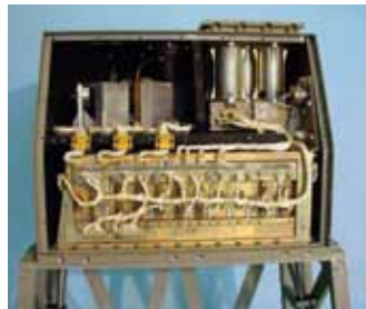
Cutaway of the Occultation Radiometer ORA.
