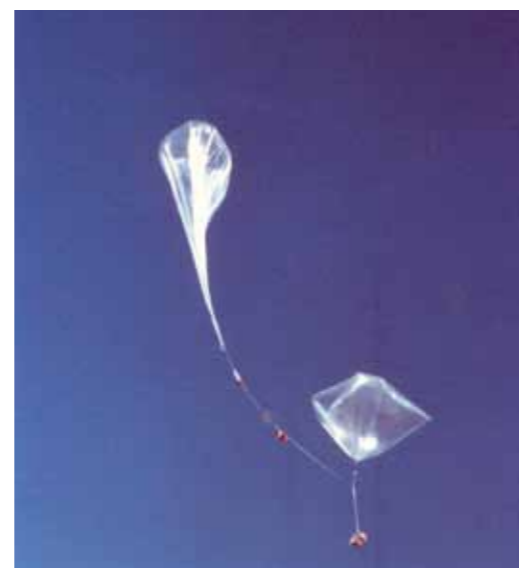
Beginning of the balloon ascent after release, the payload still hanging at the auxiliary balloon. (credit: CNES).
