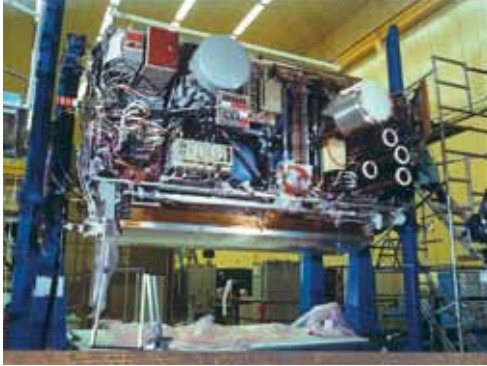
The EURECA platform developed by ESA. The ORA instrument is located at the top-left of the module next to the SOSP experiment with the red cover. (credit: MBB/ERNO)
