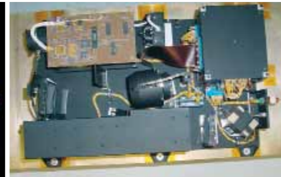
Flight Model Sensor Unit of SPICAM viewed from above. The IR acoustooptical tunable filter spectrometer is at top; the UV spectrometer is at bottom. The common optical axis points to the left. For the UV spectrometer, the light enters the mechanical baffle (black), is focused by a parabolic mirror (bottom right) through a slit, then dispersed by the grating (middle left), to be refocused on the intensified Charge-Coupled Device (CCD) Detector (at centre).
