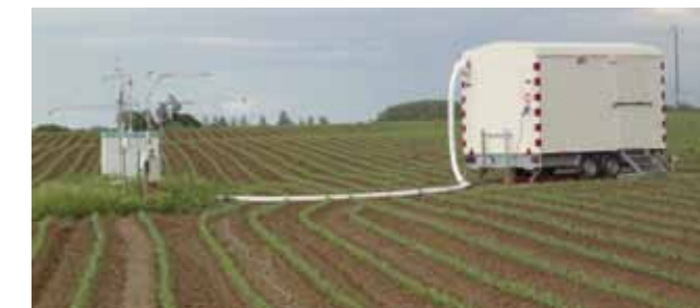
Micrometeorological measurement station and shelter, housing the Proton Transfer Reaction Mass Spectrometer and peripheral equipment, for Eddy Covariance turbulent flux measurements at a corn field at Loncée, Belgium.
