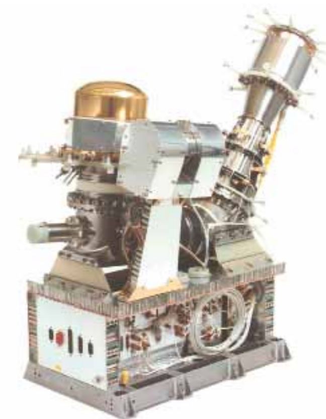
The DFMS instrument on board Rosetta, a mass spectrometer with high mass resolution. BIRA-IASB contributed to the LEDA detector and the electronics.
