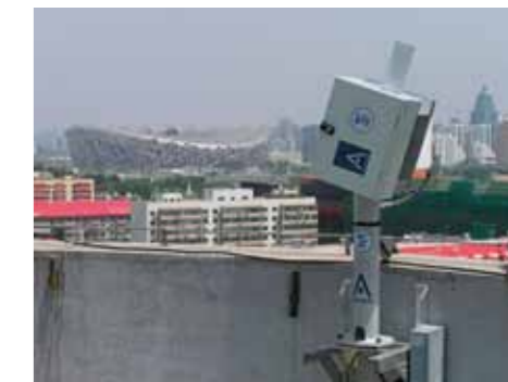
MAXDOAS instrument installed in Beijing from June 2008 to April 2009 on the roof of the Institute for Atmospheric Physics (China).
