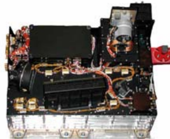
Cutaway of SOIR instrument on board Venus-Express.
