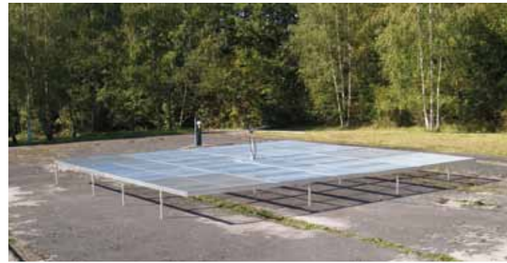
Top: Transmitter located in Dourbes (a crossed dipole with a 8m x 8m metallic grid acting as a reflecting plan). Left: Receiving antenna located in Uccle (3-elements Yagi antenna).
