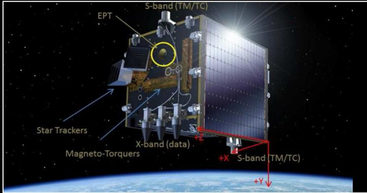
Together with UCL and Qinetiq Space, BIRA-IASB has built the Energetic Particle Telescope, carried on the Proba-V satellite in an 820 km high polar orbit, scanning the low-altitude footprint of the radiation belts.
